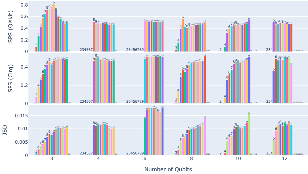
Fig. 8. Simulated Performance Scores (SPS) for Qiskit (top) and Cirq (middle), along with the Mean JS Divergence between Qiskit and Cirq (bottom). The data is grouped by the Number of Qubits, with Circuit Depth annotated above each bar.
